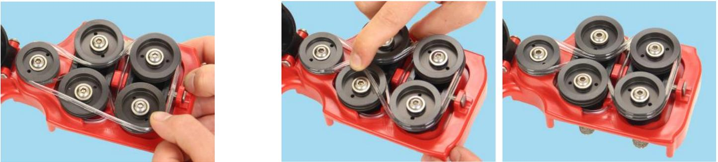
**Spindle Modules** are designed to be replaced, for easy servicing.
