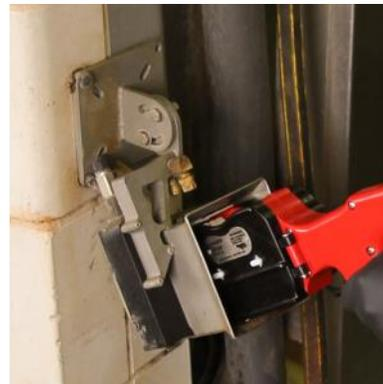
C. If you are using the extension bracket, use the provided hardware to position the holster in a ergonomic position, then tighten the extension bracket bolts.
