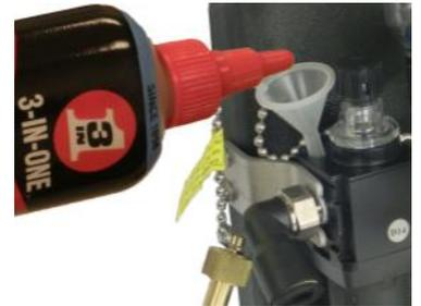
**WARNING** If the Udder Gun dose not receive enough air tool oil, the air cell will be damaged.
