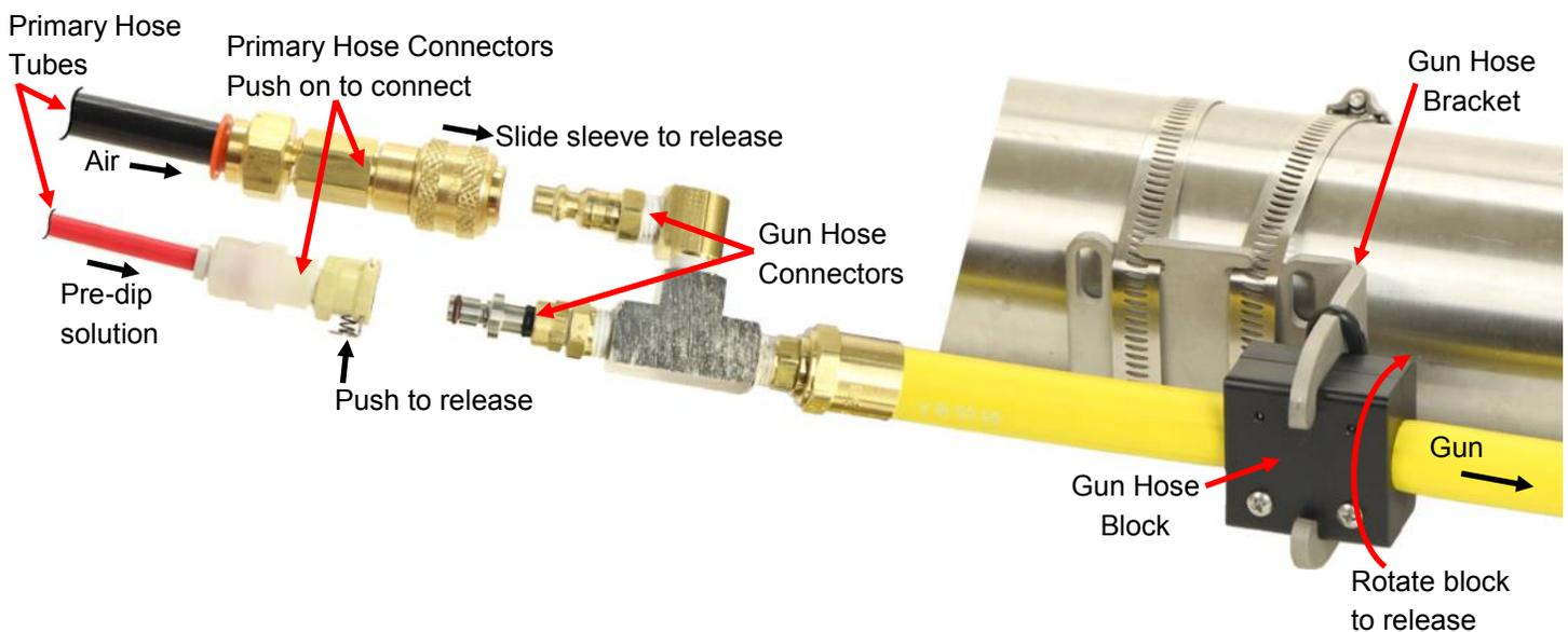
4. Lock the gun hose block onto the bracket.
