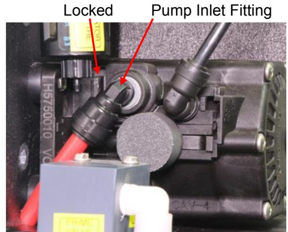
Slide to Unlock Pump Inlet Fitting
